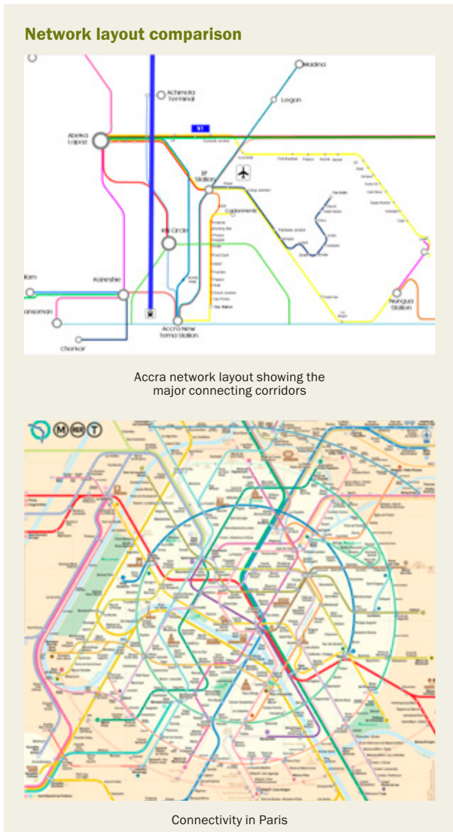
Comparison of the concentric circles of an orbital network with consistent grids in Paris with Accra's north–south orientation with only the semi-circle (ring road) providing limited east–west movement
